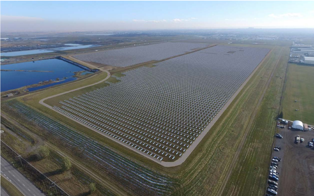
We use bifacial panels at our Barlow and Deerfoot solar projects to generate electricity from both the direct sun on the front face and the reflected sun on the back.
