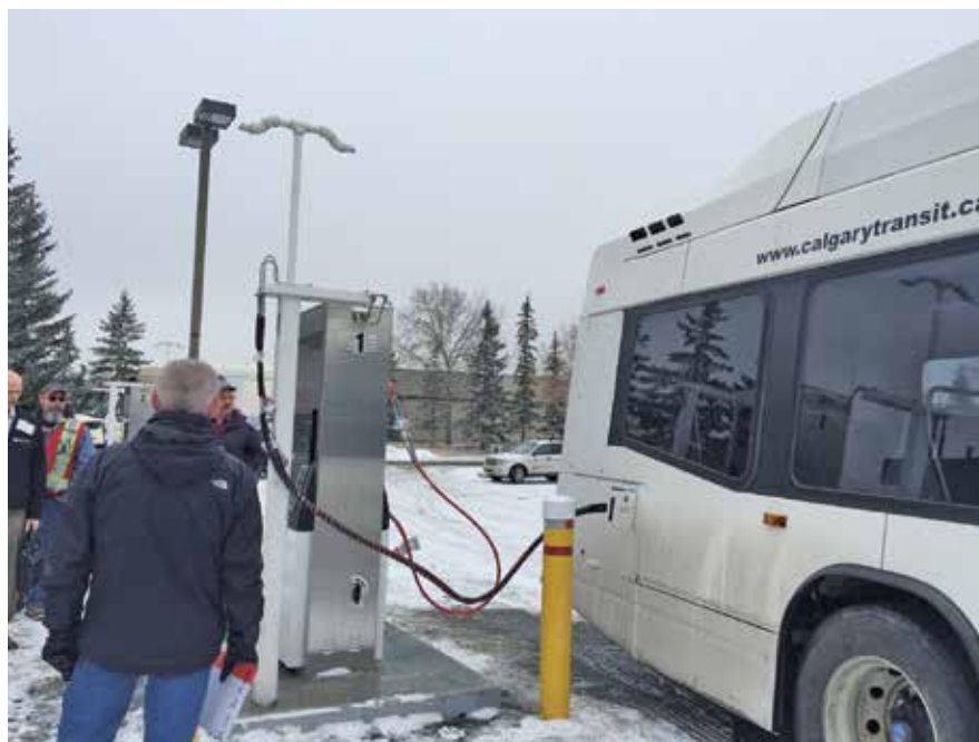
A Calgary transit bus fuels up with compressed natural gas at ATCO Gas's newly retrofitted, state-of-the-art natural gas vehicle refuelling station in Calgary.
